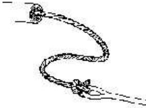
*Direct Attachment: Strength member is tied directly to the pulling fixture. The cable end must be sealed to prevent intrusion of moisture while pulling.*
