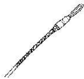
*Indirect Attachment: Pulling forces are distributed over the outer cable structure.*
